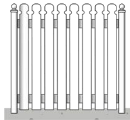
Vertical spaced boards, view
